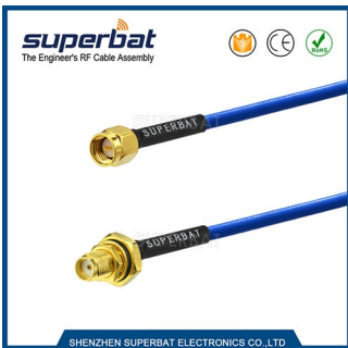
SMA Jack to SMA Plug Using Blue Jacket Coax Cable .141
